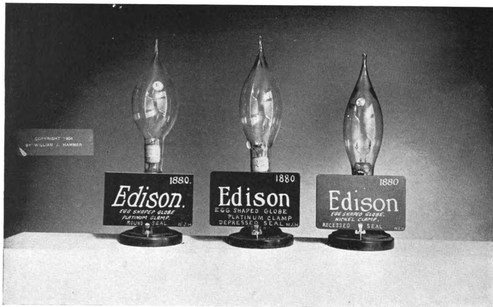
Fig. 9 Egg shaped Edison lamps with carbonized bamboo filament of 1880
