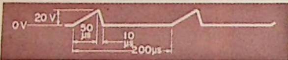
One PRF Unit, one Pulse/Delay Unit, and one Pulse Shaper with the PRF Unit set for 5 kc/s. Rise and fall times are independently variable.
