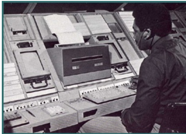
Figure 4: NAS Stage A (ca. 1973). Pictures from FAA at https://www.faa.gov/about/history/photo_album/air_traffic_control . Above is Plan View Display (PVD) in En Route sector position. The original PVDs could be rotated horizontally to accommodate backup (digital channel failure) “shrimp boat” markers of flight identification. Below is the Computer Update Equipment (CUE) for sector participation in Flight Data Processing (FDP) but with paper flight strip interface visible in the strip bay behind the controller's head.
