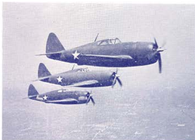
Republic P-47 Thunderbolt Produced for U. S. Army Air Forces, Equipped with 2000 hp. Pratt & Whitney Engine, Turbo-Supercharger and Many Electrical Devices
