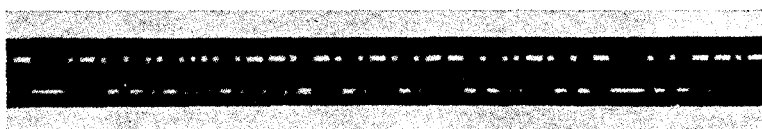
Fig. 6. Reception of wireless signals from an arc transmitter with two galvanometers. The string of one is tuned to the working wavelength and that of the other to the wavelength used when not transmitting signals. Whilst one string oscillates the other remains quiescent and vice versa.
