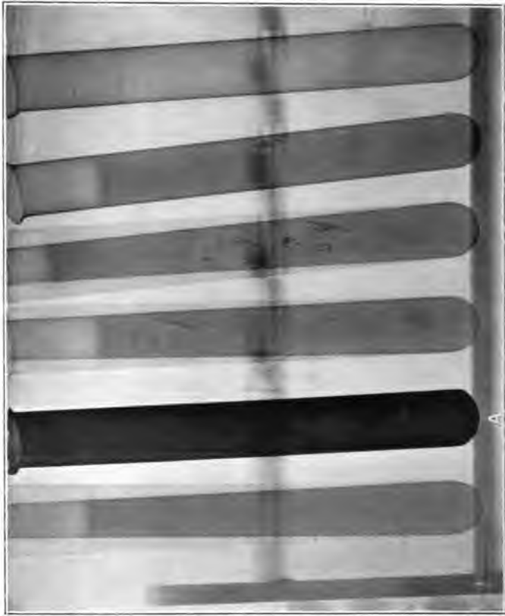
FIG. 3.—[ILLUSTRATING ABSORPTION OF RONTGEN RADIATION BY FLUORESCENT LIQUIDS OR FLUORESCENT COMPOUNDS, TUBES, ETC.]
