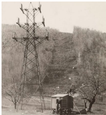
Equipment for cathode-ray oscillographic study of surges on transmission line from Turner Falls, Mass. Impulse generator applying surges on transmission line at Ferncliff Tower located 5.77 miles from Pittsfield, MA.
