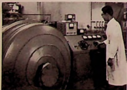
Wesgo vacuum processing furnace for oxide free brazing alloys
