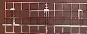
FEW Pulses as few as 2.5c/s, or single pulses using accessory trigger.
