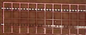
MANY Pulses up to 1.2 Mc/s internally or to 2.2 Mc/s with external drive.
