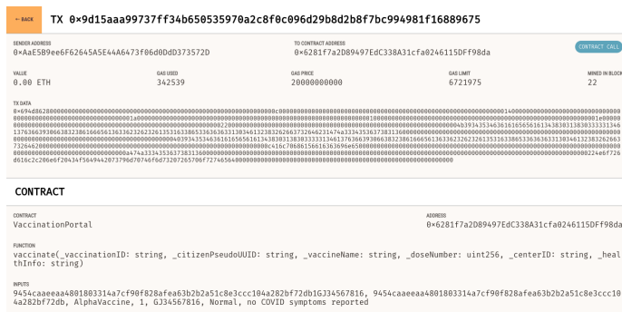
Fig. 12. Data for the transaction which registered a new vaccination for a citizen
