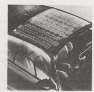
Solar cells continuously power electric ventilation.
