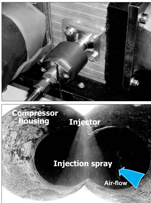
Figure 15 Water injection into the compressor [9]
