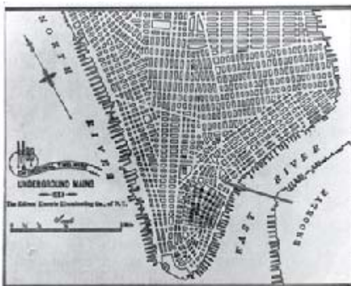
figure 2. Map of lower Manhattan showing the original area served by the Pearl Street station and its distribution system (courtesy of the Consolidated Edison Company of New York).
