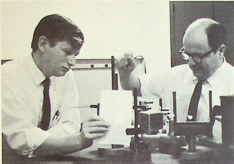
Wright Huntley (left), and Dominic DeSimone (right), adjusting pinhole spatial filter preparatory to making a hologram.
