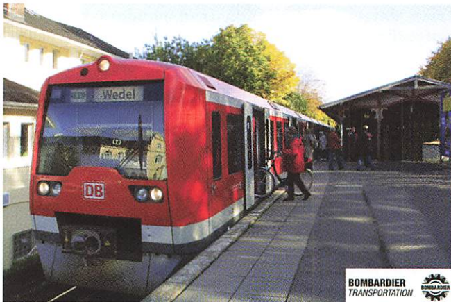
Type 474 Unit for the type being rebuilt as dual voltage
