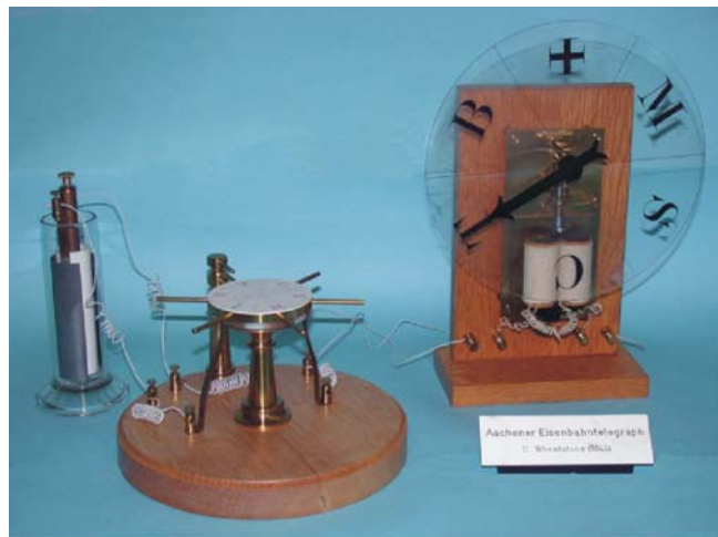
Fig. 2: Aachen Railway Telegraph 1843
