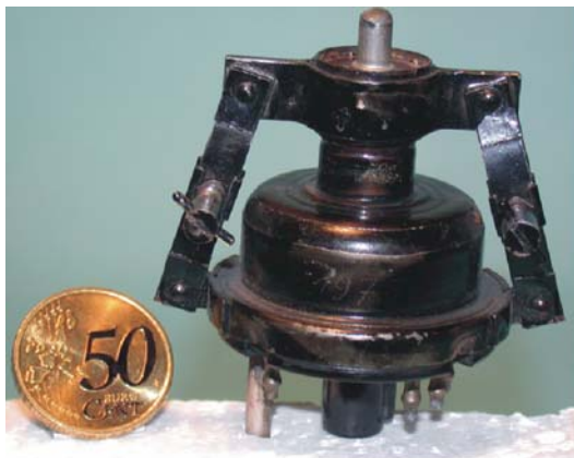
Fig. 15: Low power Reflex-Klystron, 1944
