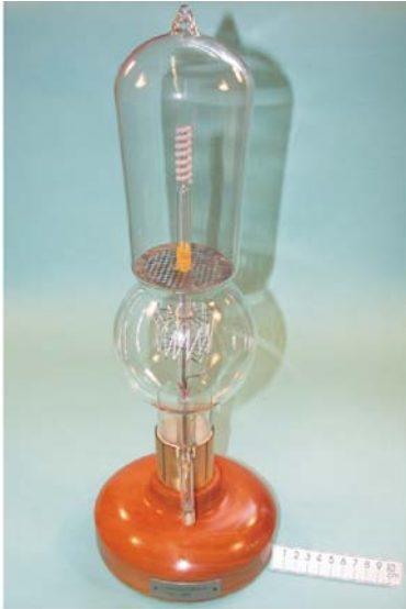
Fig. 4: Replica of v. Lieben tube, 1908
