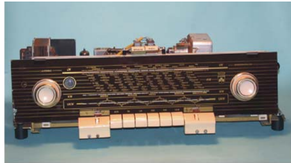
Fig. 9: Superhet-radio with magic eye, 1950
