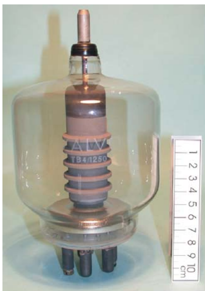
Fig. 14: High power transmitter Triode, 875 W, 1980
