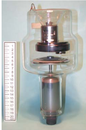
Fig. 12: X-ray tube with rotating anode
