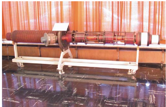
Fig. 16: 600 kW multi cavity Klystron, 500 Mhz
