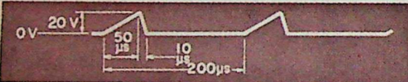
One PRF Unit, one Pulse/Delay Unit, and one Pulse Shaper with the PRF Unit set for 5 kc/s. Rise and fall times are independently variable.
