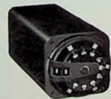
Coaxial Synchro Standards. Ideal where panel space is limited. Occupies only 2 1/4" square panel area. Outer dial switches in 60° increments; inner dial in 5° increments. Zero to 360° range. 2 seconds-of-arc accuracy.
