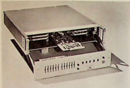
Front access "card cage," Dymec division of Hewlett-Packard Co., Palo Alto; Gerry Priestley; Bob Pierce, Arlan Saunders, Ted Pollard.
