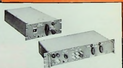
Synchro Standards or Resolver Standards. One-knob or two-knob models available as either synchro or resolver standard, in half rack or full-rack size. Continuous angular rotation from 355° to 0°, in 5° increments. 2 seconds-of-arc accuracy.
