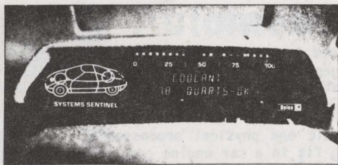
Buick Questor Heads-Up Steering-Column-Mounted Display
