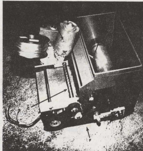
Prototype On-Board Hydrogen Generator (A - Aluminum Wire; B - Wire Feed Motor, C - Carriage Traverse Screw; D - Rotating Drum In Water Tank; E - Wire Guide Tube; F - Tooth belt Driven By Underside Motor Driving Screw And Drum)
