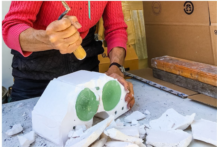
The glass insulators for the legs of the diodes and transistor were made using the lost wax kiln cast process and Bullseye Glass.
