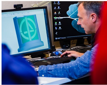
The CAD software at Nor-Cal allowed us to scale up these 18' tall sculptures. The shop drawings they produced were used to cut and assemble the steel pieces.
