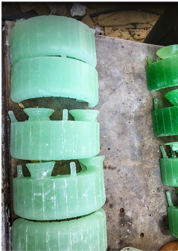
The glass insulators for the legs of the diodes and transistor were made using the lost wax kiln cast process and Bullseye Glass.
