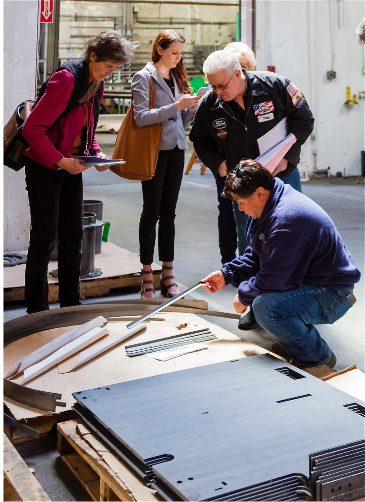
The CAD software at Nor-Cal allowed us to scale up these 18' tall sculptures. The shop drawings they produced were used to cut and assemble the steel pieces.
