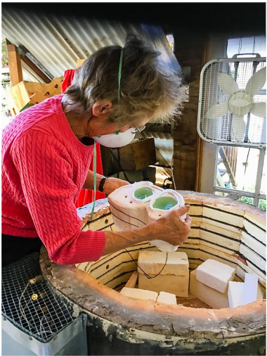
The glass insulators for the legs of the diodes and transistor were made using the lost wax kiln cast process and Bullseye Glass.
