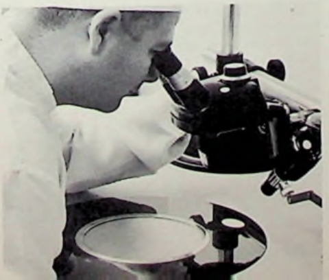
Quality Control Laboratory. Each coated disc must pass a thorough examination. Here we conduct a microscopic check for any surface errors.
