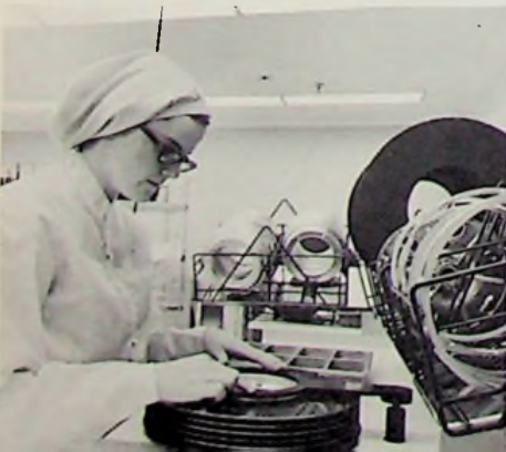
Pack Assembly. A memorex employee carefully assembles disc into a pack. The completed disc pack will undergo thorough QC tests before it is released.
