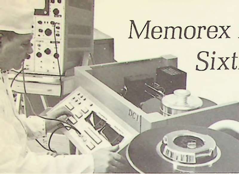
Disc Certifier. At special certifiers designed by Memorex, each individual disc is checked to insure against any surface errors. Any error is cause for rejection of entire disc.
