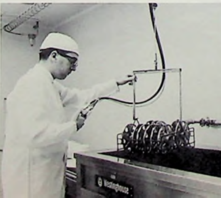
Ultrasonic Cleaner. All component parts of Memorex Disc Packs are ultrasonically cleaned to remove microscopic particles that cannot be visually detected.
