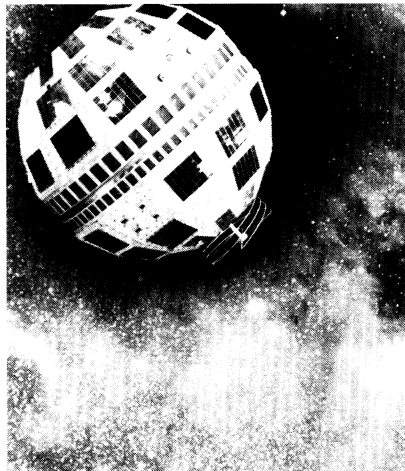
Telstar I, launched in 1962, showed the possibilities for sending telephone calls and television broadcasts across oceans and continents via an orbiting satellite
