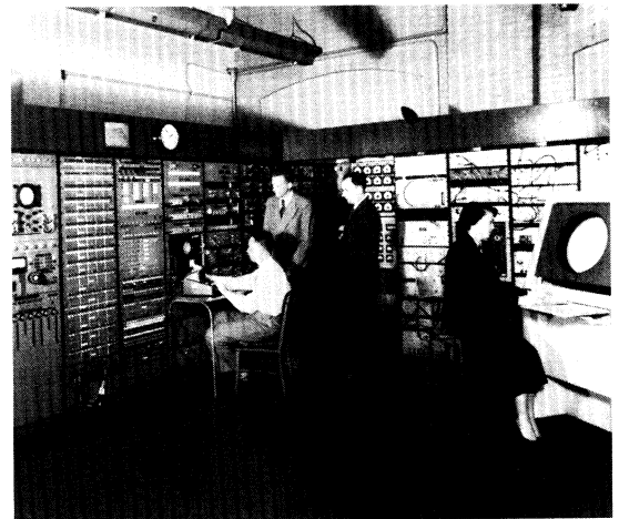
Whirlwind computer, built at MIT with Navy and Air Force funding in late 1940s and early 1950s MIT Museum
