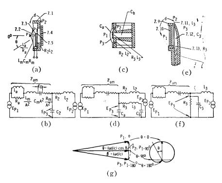
Fig. 7. Phase-shift unidirectional microphones.
