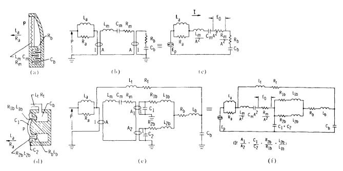
Fig. 4. Pressure microphone with velocity-responsive transducer.
