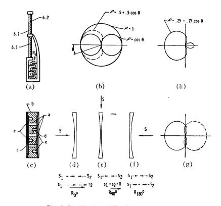
Fig. 6. Combination unidirectional microphones.
