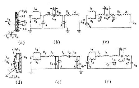
Fig. 3. Pressure microphone with displacement-responsive transducer.
