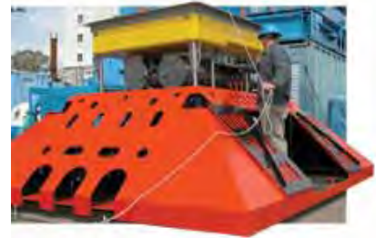
A Neptune worker lowers a scientific instrument node into its orange support frame.
