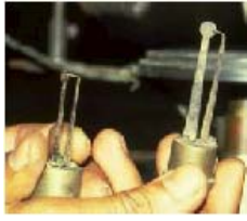
Figure 6: Two of Bose's point contact detectors, removed from the receiving antennas.
