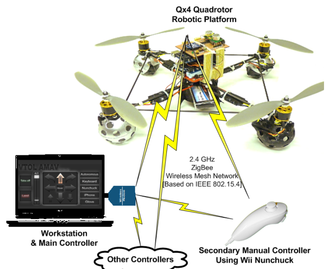
Fig. 1. System overview – system components.
