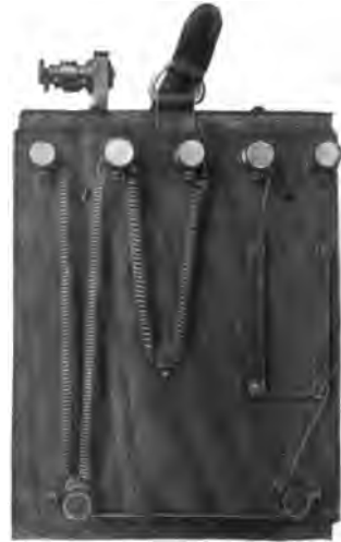
FIG. 5. PORTABLE STORAGE BATTERY FOR METER TESTING.
