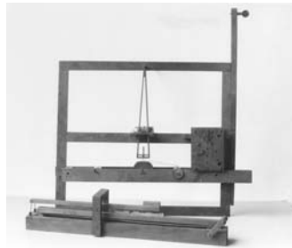
Morse transmitter and receiver (Courtesy of Smithsonian Institution)
