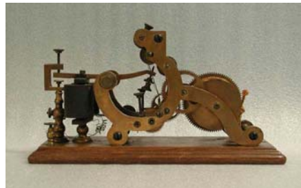
Telegraph Register by Williams, Boston (Courtesy of Smithsonian Institution)
