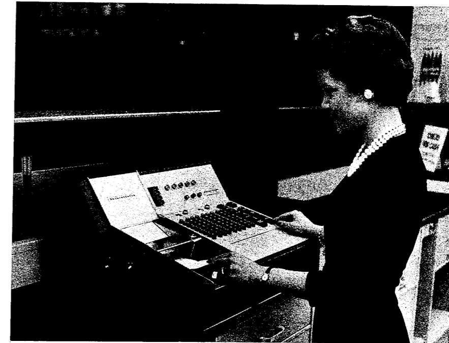
Fig. 1. The Teller-Register, an important part of The Howard Savings Institution's on-line banking system, brought about considerable improvement in customer service. This teller posting machine was designed specifically for on-line, real-time data processing as opposed to an adaptation of a conventional window machine.
