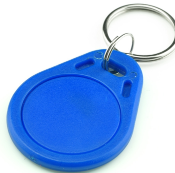
Fig. 3. Passive keychain tag
