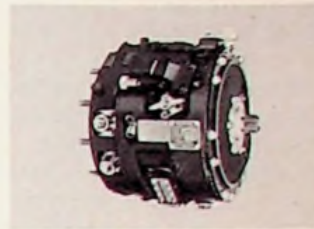
Constant speed drive similar to those installed on F-111, C-5A, DC-9, F-4, and 737 aircraft.
