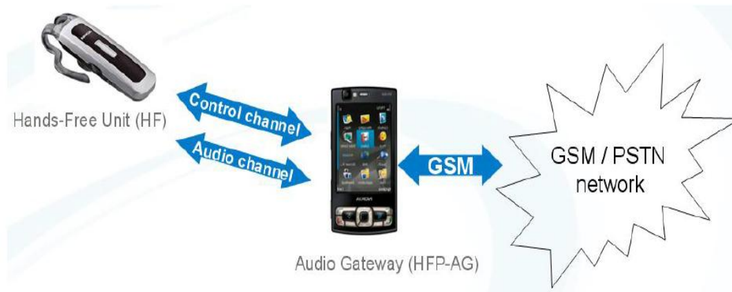
Figure 4: Bluetooth channels in a typical wireless headset
