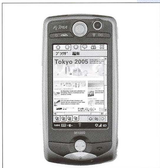
NTT DoCoMo's M1000, combining 3G (W-CDMA), 2.5G (GPRS), 2G (GSM) and WLAN in a single handset. See our discussion on Page 3. (Photo NTT DoCoMo)
