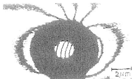
FIG. 5. Leakage fields from a toroidal magnet (phase amplification, 2\times ). Leakage flux can be quantitatively measured since a constant flux of h/2e flows between two adjacent interference fringes.
