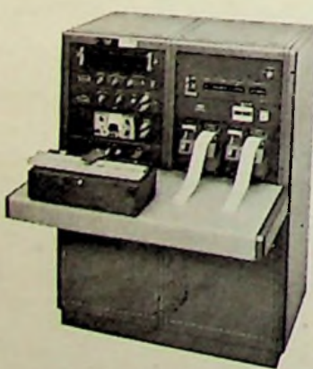
An automatic capacitor-test system produced by General Radio.
