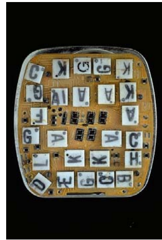
Pulsar module, 1972. Inside the Hamilton Pulsar wristwatch was this electronic module.
