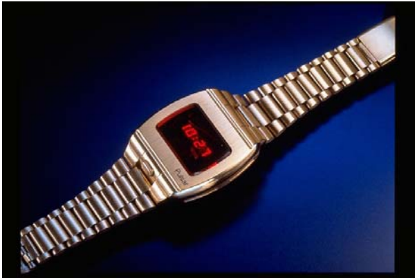
Hamilton Pulsar wristwatch with LED (light emitting diode) digital display, 1972.
