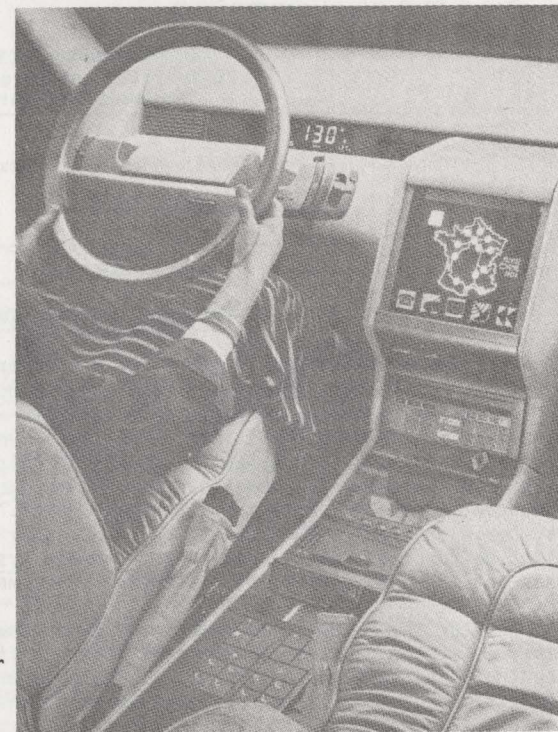
Renault Dialog Instrumentation Includes Multifunction CRT, Cordless Telephone, and Compact Disk Player
