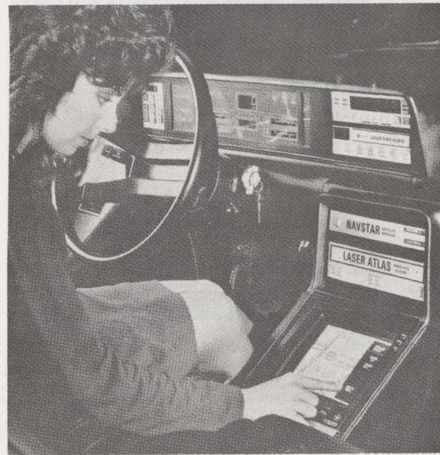
Chrysler Laser Atlas and Satellite System Which Uses a Color TV Monitor and Includes an Electronic Compass and 12-Function Navigator
