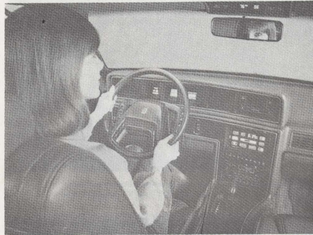
Ford Motor Comtech Instrumentation System Which Includes Steering Pod Mounted Multiplex Control
