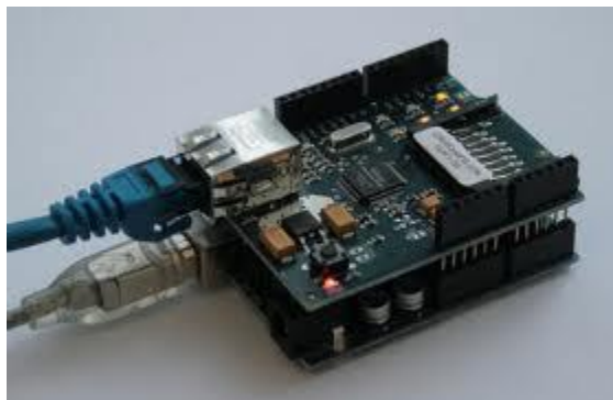
Figure 2 Arduino Ethernet Shield which provides the web connection to patient's MCU
