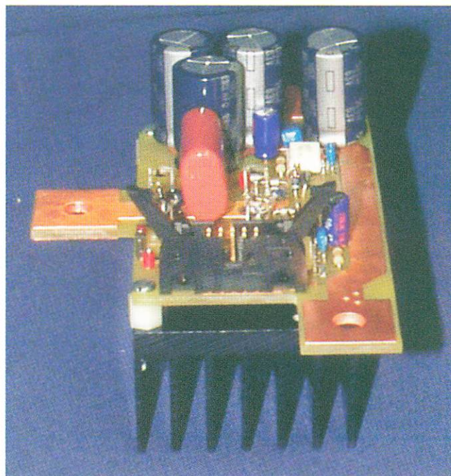
Figure 3 140A/60V (2kW) multilevel cell w/ self-powered gate drive
