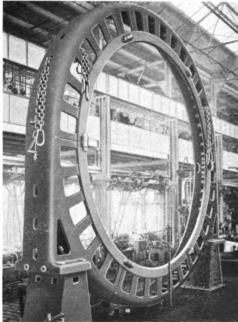
Stationary Armature Frame of 3500 Kw. Three-Phase Alternator
