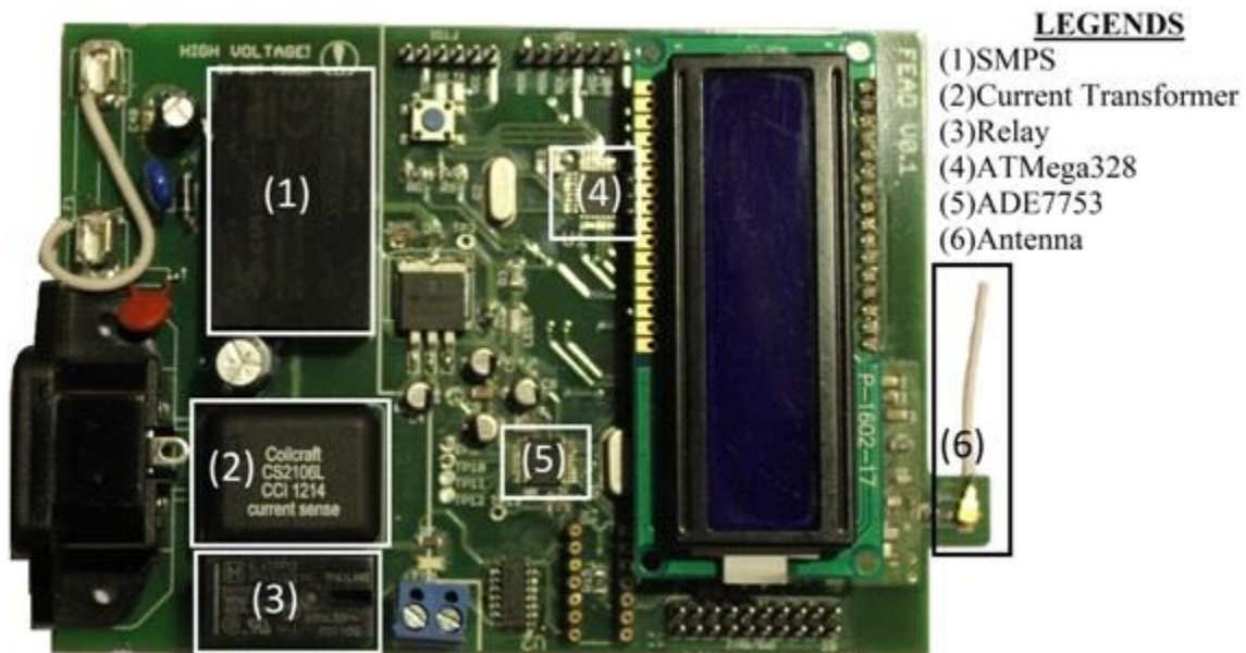
Figure 9: Energy Metering Node
