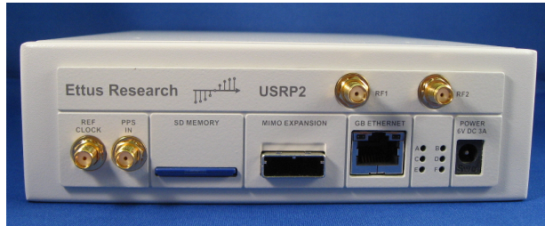
Fig. 2: Ettus Research Universal Software Radio Peripheral 2 (USRP2)
