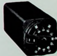
Coaxial Synchro Standards. Ideal where panel space is limited. Occupies only 2 3/4" square panel area. Outer dial switches in 60° increments; inner dial in 5° increments. Zero to 360° range. 2 seconds-of-arc accuracy.
