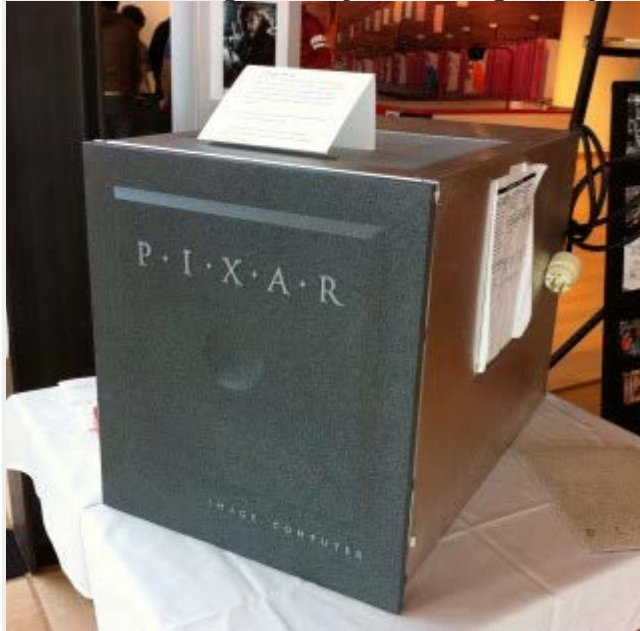
A Pixar Image Computer. (One sits now at the front of Pixar's internal renderfarm in Emeryville, CA)
