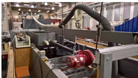
Figure 5 VFD Verification Testing Set Up
