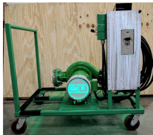
Figure 7 Completed Pumping Solution Cart and Control Box
