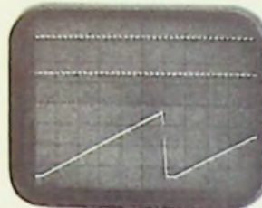
Either half of the split-screen can be used for a stored display, the other half for a nonstored display. (Shown below).
