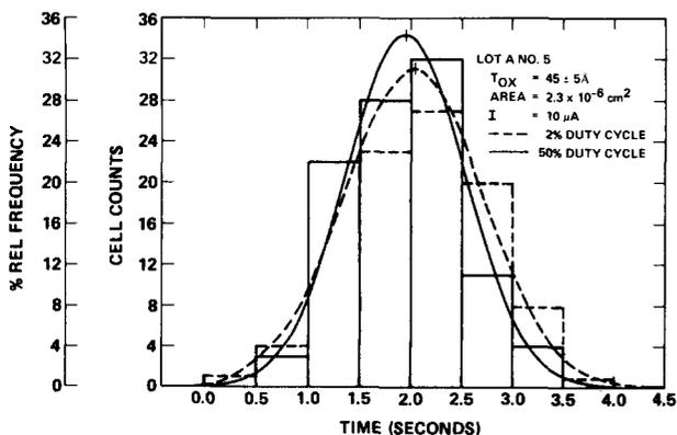
FIG. 9.  $T_{BD}$  distributions at 2 and 50% duty cycle constant current pulsing.
