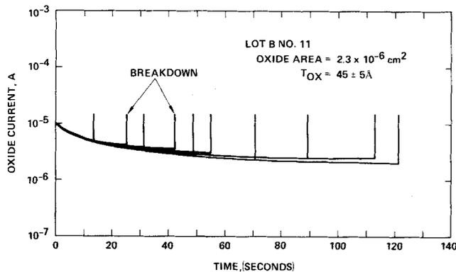
FIG. 3. Measured time to breakdown for thin-oxide samples stressed at a constant gate voltage.  $T_{BD}$  at constant  $V_g$ .
