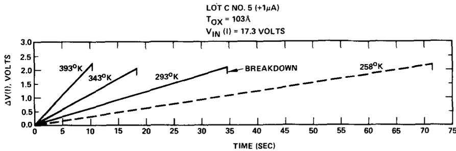
FIG. 13. Change in  $V_{in}(I)$  as a function of time under constant current stress at various temperatures.
