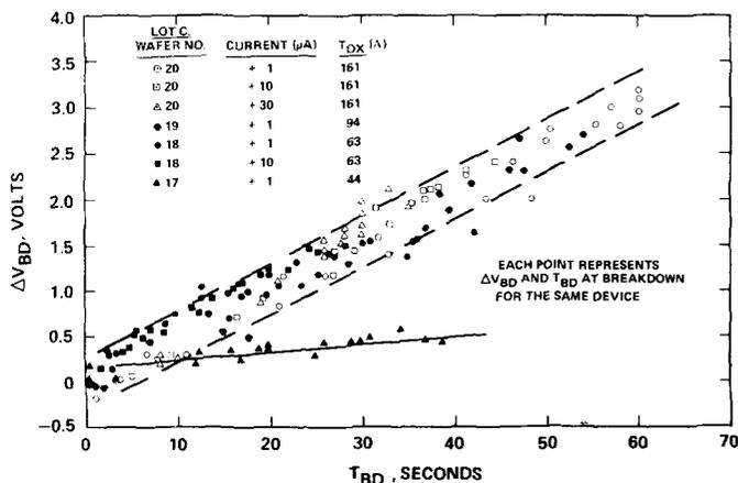
FIG. 7. Relation between  $\Delta V_{BD}$  and  $T_{BD}$  for individual samples of different thicknesses. All  $T_{BD}$  values are normalized to a +1- $\mu A$  current level by assuming  $T_{BD}(I) = \text{const}$ .
