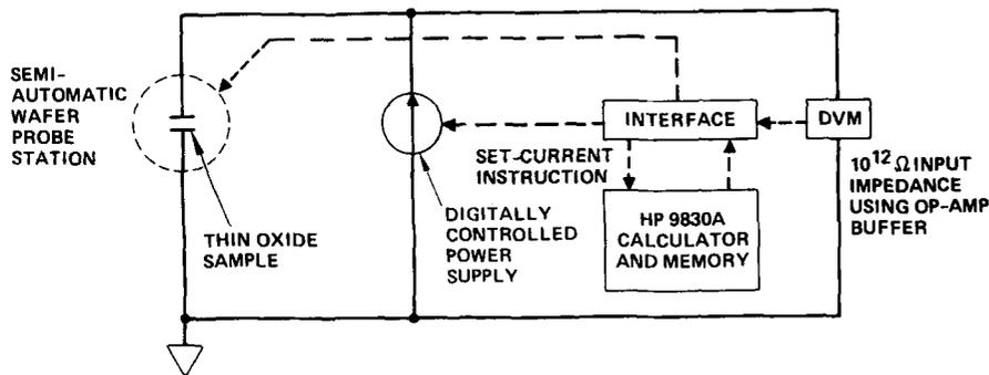
FIG. 1. Automated experimental setup. The required current level is set into the program. The computer prints out and stores the following data: (1)  $V_{in}$  (V) at set current, (2)  $T_{BD}$  (sec) at set current, (3)  $\Delta V_{BD}$  (V) at set current.
