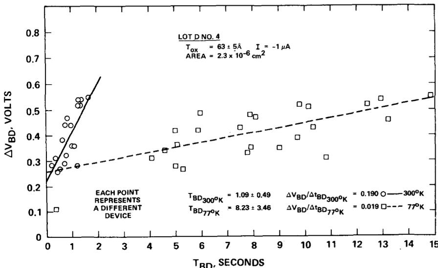
FIG. 12. Relation between  $\Delta V_{BD}$  and  $T_{BD}$  for individual samples stressed under identical conditions at either  $77$  or  $300^\circ\text{K}$ .
