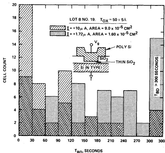
FIG. 4. Effect of area of stressed oxide on the  $T_{BD}$  distribution (at constant current density).
