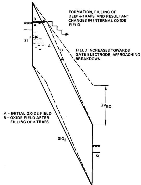
FIG. 15. Buildup of internal fields due to generation and filling of electron traps close to the injecting electrode.
