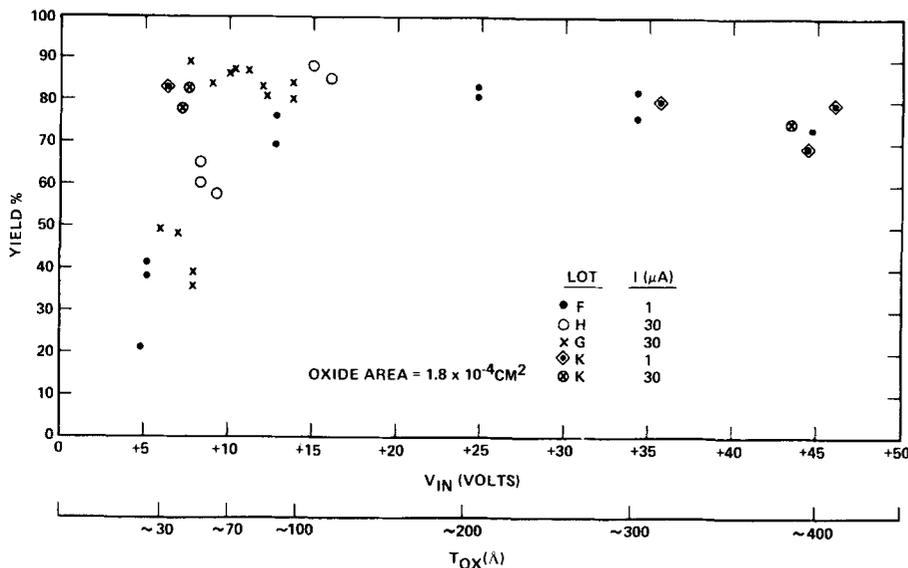
FIG. 14. Yield as a function of oxide thickness for batches of oxide capacitors stressed at constant current.
