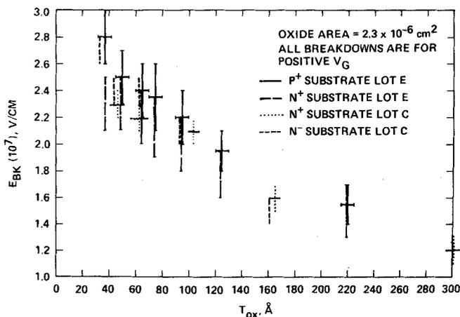
FIG. 5. Oxide breakdown strength for ultrathin oxides as a function of oxide thickness. All data shown for positive  $V_g$ . Negative  $V_g$  breakdowns are lower by 5–10%.
