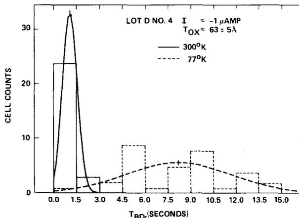
FIG. 10.  $T_{BD}$  distributions at 77 and 300°K with otherwise identical conditions.
