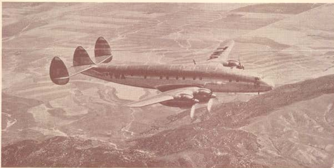
Lockheed C-69 "Constellation" now in production for the Army Air Forces. This is an all-range, high-performance transport, which broke all transcontinental records when flown from Burbank to Washington in 6 hours and 58 minutes at an average speed of 330 miles per hour.
