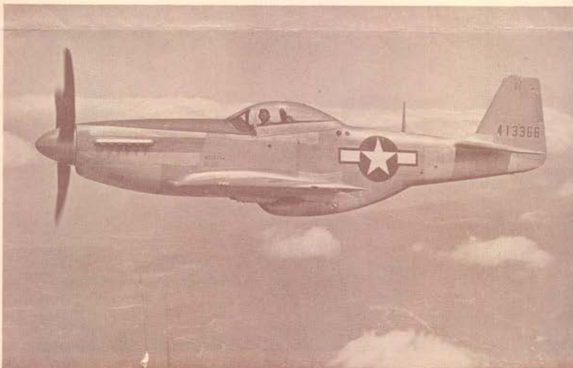
The North American P-51 Mustang with new "teardrop" cockpit enclosure affording complete vision in all directions
