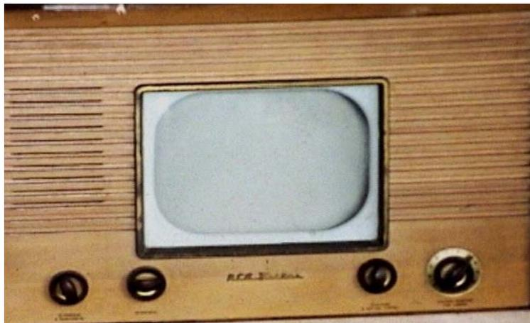
These early display tubes needed an Ion Trap to keep the heavy ions from the filament from discoloring the center of the phosphor display. Strategic investments in Ion Trap manufacturing plants didn't pan out as shortly a little trick known as the "straight gun" for the CRT eliminated their future requirement.
