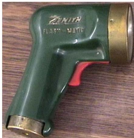
In the 60's most remotes were controlled ultra-sonically with tuning bars tapped like a piano sending signals in the range of 20 KHz. The clinking of change in your pocket or a dog's metal collar would frequently be enough to change the channel!
