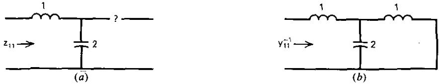
Figure 3.6. Network realizations for Example 3-14 using (a) z_{11} (or z_{22} ) and (b) the reciprocal of y_{11} .
